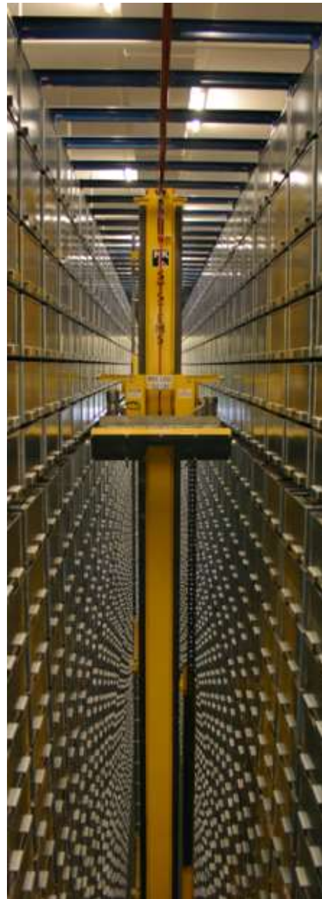
Intérieur de l'Automated Storage and Retrieval Service (ASRS), University of British Columbia
